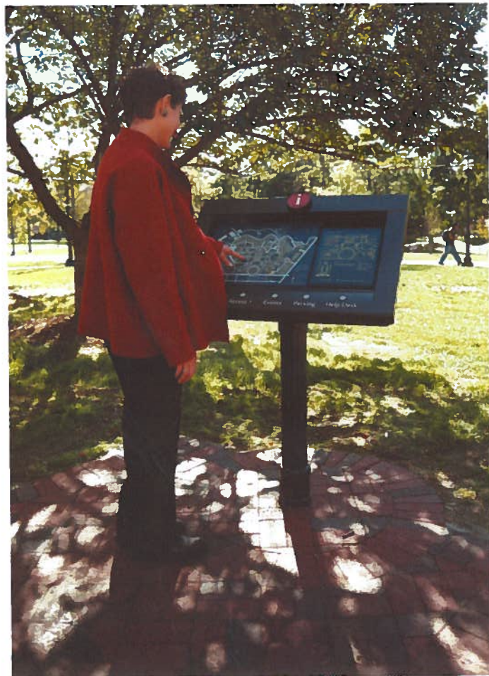
ABOVE: The anodized aluminum map works like a conventional, static map but is also interactive. The map panel sits below a grid of infrared beams. When a finger touches the map the beam is interrupted, activating the LCD screen.
